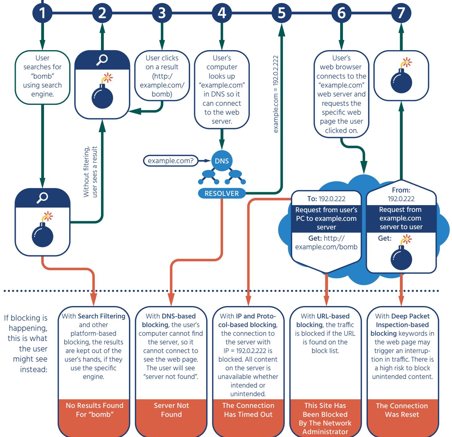
Of course, the Internet is much more than search and web browsers, and many of the techniques discussed below are effective at blocking more than web pages. For example, use of VPN services to encrypt and hide traffic can often be blocked using a combination of Deep Packet Inspection-based blocking and IP/Protocol-based blocking.
