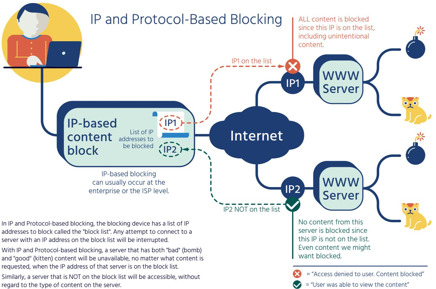
In IP and Protocol-based blocking, the blocking device has a list of IP addresses to block called the "block list". Any attempt to connect to a server with an IP address on the block list will be interrupted.
