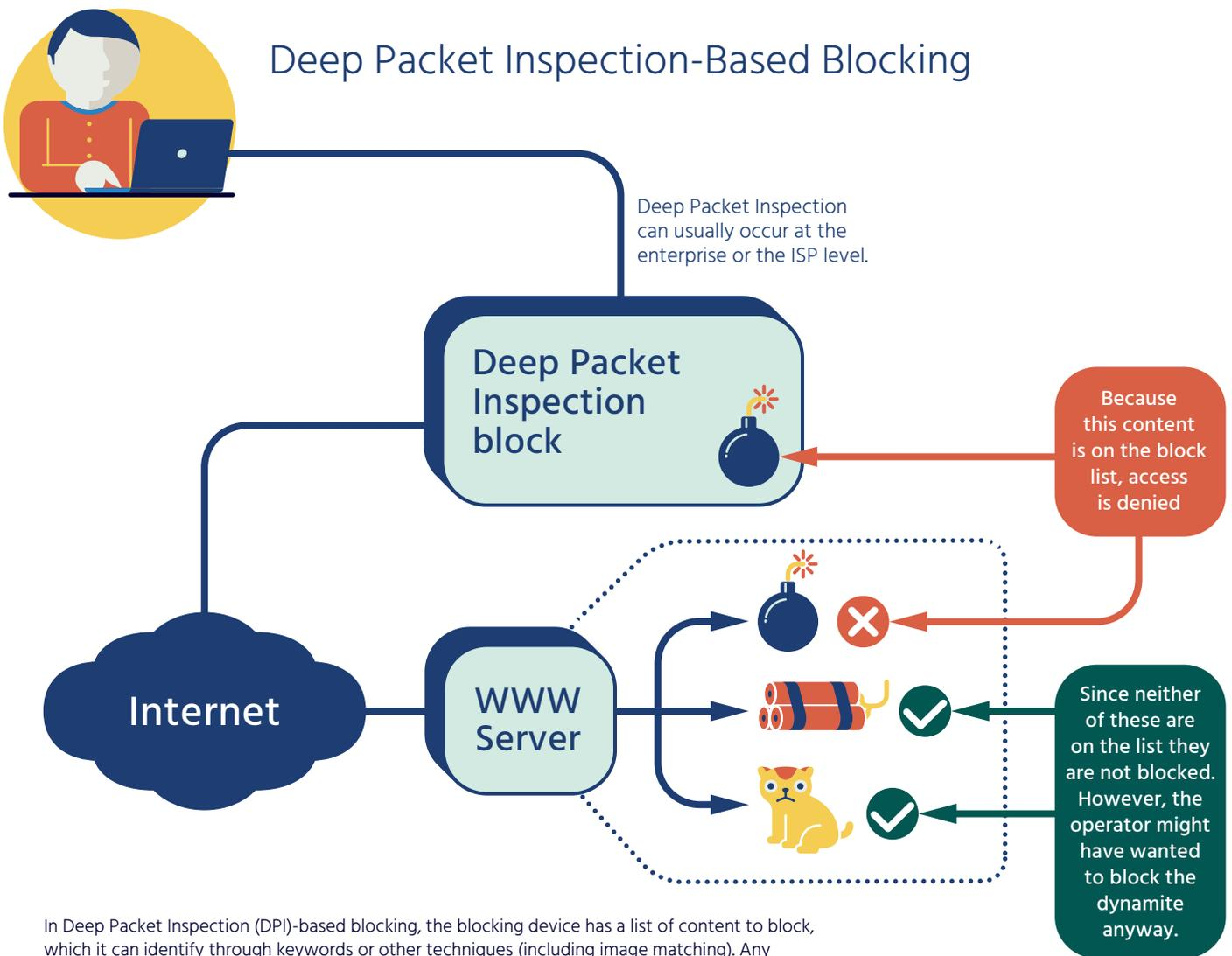
In Deep Packet Inspection (DPI)-based blocking, the blocking device has a list of content to block, which it can identify through keywords or other techniques (including image matching). Any attempt to download unencrypted content that matches the list will be interrupted.
