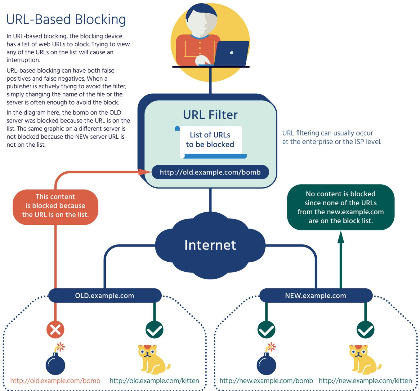
URL blocking requires the blocking party (such as the user’s ISP) to have the ability to intercept and control traffic between the end-user and the Internet. URL blocking is usually expensive, because the filtering device generally has to be in-line between the user and the Internet, and thus requires a high level of resources to give acceptable performance.
